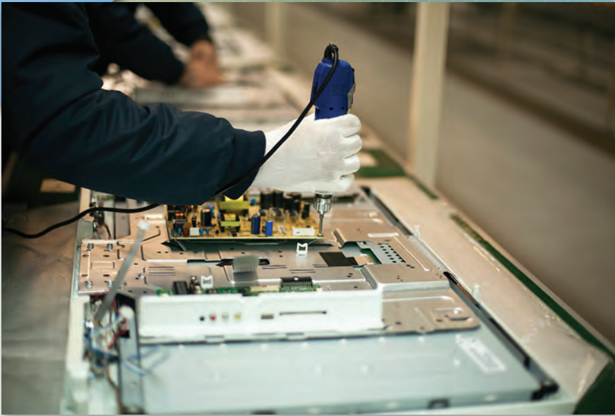
Characteristics of good production methods include having tools and materials close at hand for line workers and one-piece flow with no batching.
